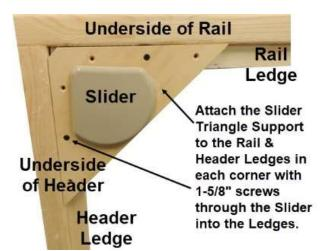
Attach the Triangle Support Slider underneath the frame with 1-5/8" screws into the four corners.
