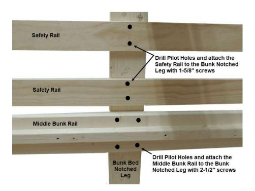
Attach the Middle Bunk Rail & Safety Rails to the Bunk Bed Notched Leg.
