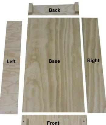
The drawer pieces include the Base, Front, Back, Left and Right sides. The Front & Back have the 2x2 support blocks already installed.
