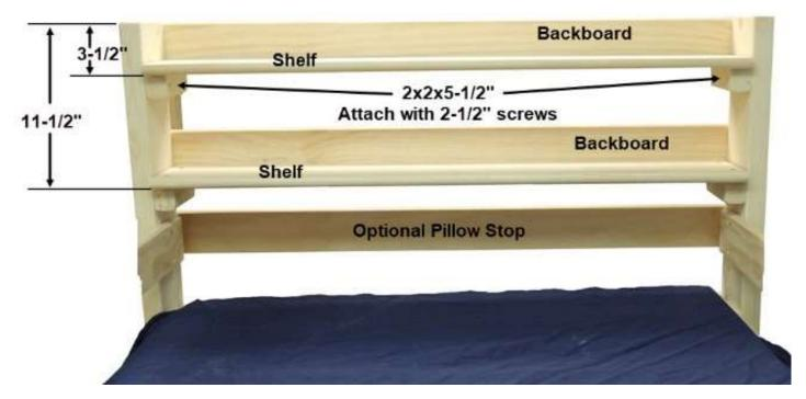
Install the Backboards to the back of the shelves. Use 1-5/8" screws at the ends when screwing into the Legs and 1-1/4" screws when screwing into the shelf.
