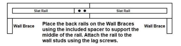
Next place the back rails along the wall and attach the rail to the wall using the lag screws using the same method as the Support Braces on page 1 and 2 of the Loft / Bunk Beds Attached to a Wall Assembly Instructions.
