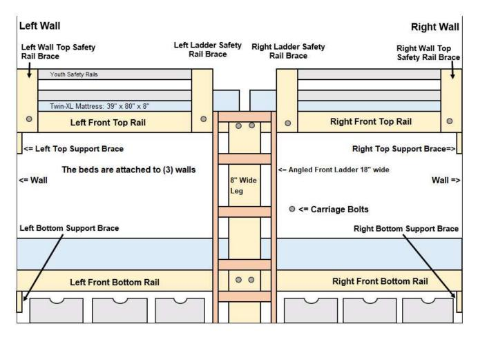
This set of instructions covers the additional steps needed to assemble the bed to Three Walls.
