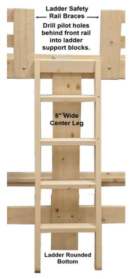
The Angled Front Ladder comes preassembled. Place the ladder between the Safety Rail Braces. The ladder has support blocks mounted on each side so it can rest against the 8" wide leg. Drill (3 - 4) pilot holes from behind the Front Rail, spacing them 3" -4" apart to line up with the support blocks of the Angled Ladder. Attach the Ladder from behind with 2-1/2" screws.
